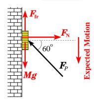
**Solution:** The free-body diagram for the book is shown: (i) The normal force  $F_N$  is normal to the contact surface, (ii) The force, Mg (due to gravity) is downward and (iii) since the expected motion (if  $F_P$  is not sufficient) is downward, the force of friction  $F_{fr}$  is upward.
