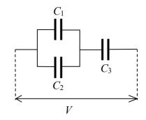
4. An air-filled parallel-plate capacitor with a plate area A and separation d, has capacitance  $C_0$ . Then, the capacitor is partially filled with three dielectric slabs with constants  $K_1 = 4$ ,  $K_2 = 5$ ,  $K_3 = 6$ , as shown. Each dielectric slab fills 1/3 of the space between the capacitor plates. If the equivalent capacitance is 200 µF, find the initial capacitance  $C_0$ . [5 points]
