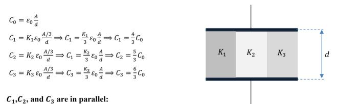
$C_{eq} = C_1 + C_2 + C_3 \Longrightarrow C_{eq} = \frac{4}{3}C_0 + \frac{5}{3}C_0 \frac{6}{3}C_0 \Longrightarrow C_{eq} = \frac{15}{3}C_0 \Longrightarrow C_0 = 40 \ \mu\text{F}$
