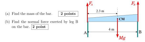
Solution: The free-body diagram is shown. We choose the **pivot at the right-end** of the bar. The net torque on the bar about this pivot is
