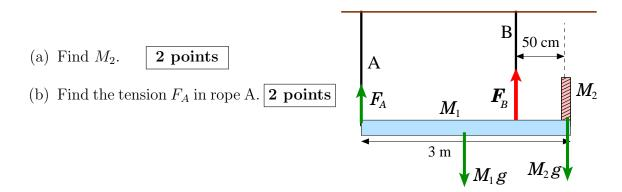
Solution: The free-body diagram is shown. We choose the pivot at the point where the rope A is attached to the bar. Then the net torque on the bar is,
