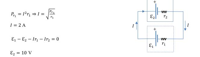
7. In the circuit shown, calculate the potential difference  $V_{ab}$
