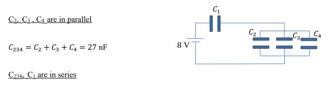
$$C_{eq} = \frac{C_1 \times C_{234}}{C_1 + C_{234}} \Longrightarrow C_{eq} = 6.75 \text{ nF}$$
